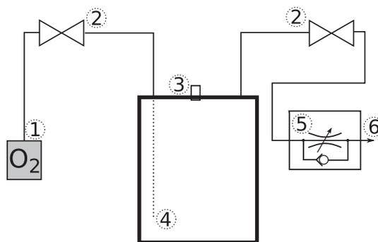
**FIGURE 2** Sketch of the reactor used. 1: (99%) Oxygen bottle with valves; 2: shut-off valve; 3: septum for fluid handling; 4: tube glued to the bottom (optional); 5: throttle check valve; 6: gas outlet
