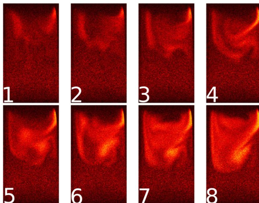
**FIGURE 3** Visualization of gas ingress to a acetonitrile solution of [Cu(btmgp)I] with an image separation of 14.45 s
