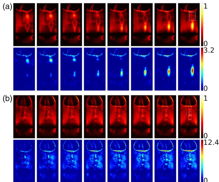
**FIGURE 4** Monitoring the rise of one bubble and the reaction in its tail. One image was acquired every 3.2 s. In the top row, the raw spin density images are depicted whereas in the bottom row the calculated relative concentration maps are depicted. The invisible area on the bottom in the top row is an artifact from the birdcage resonator. The oxygen flow rate in (b) was decreased compared to (a)
